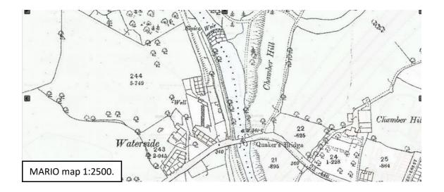
The diverted water became the mill race and supplied the mill pond. The pond has been filled in and all that remains is a depression in the field. There is an overflow shown on both MARIO maps; presumably this was an open stream. What happened to the water used in the factory is not indicated on the maps – assumed returned to Pendle Water via an underground drain.
